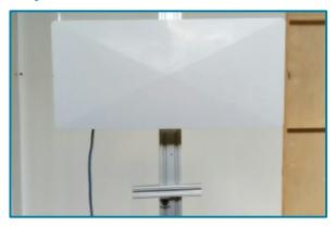
As you would for any RAIN RFID application, test the read zone of the xSpan. Verify that the read zone meets your needs. For example, place your tagged items as close as possible to the xSpan while still on the ground so that all the tags still can be read as show in Figure 16.
