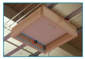
• The best way to mount in a grid system is to line up the ground plane of the xArray with the Grid System. The ground plane is 1" from the face of the radome (2 inches from the backplane). Figure 12 features a side view for demonstration.
