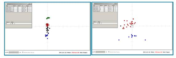
Location Mode for items on bottom shelf when unobstructed (left), vs. when the read is obstructed by shelving (right).
