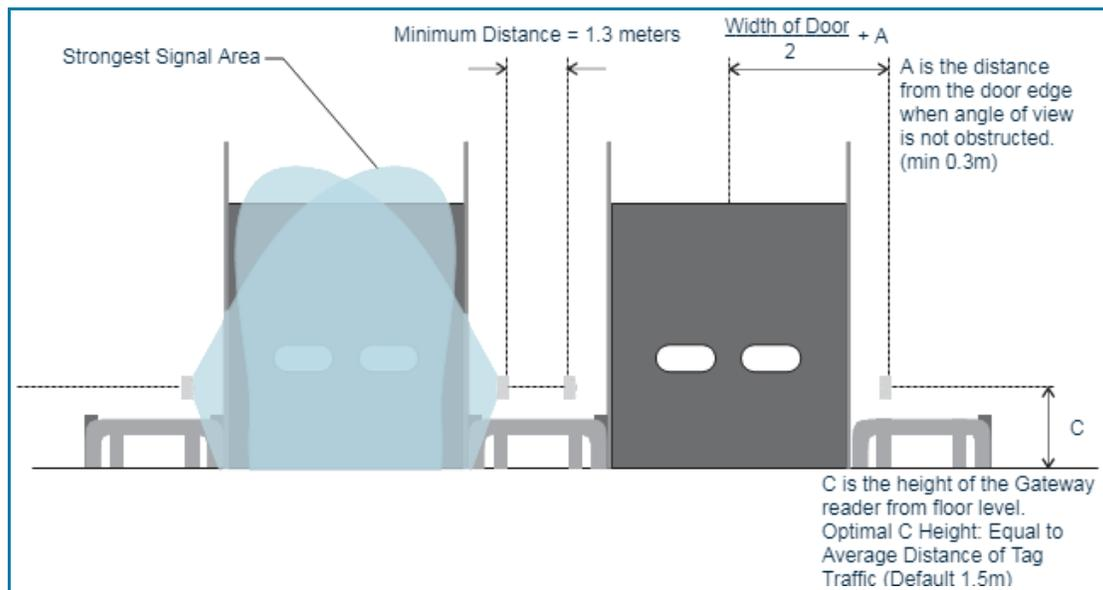
*A typical dock door side-by-side reader setup, with recommended dimensions.*
