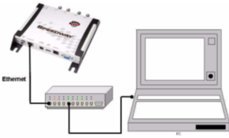
Figure 5.4 Connecting the Speedway Reader to the Ethernet Network
