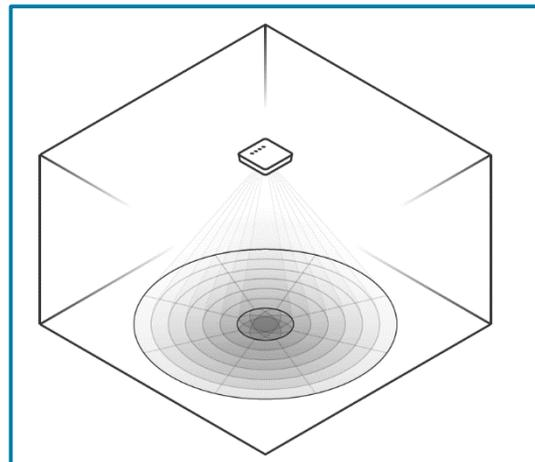
For the xSpan, enabling all 13 antennas provides an oblong 3 dB beamwidth coverage area approximately 120° major axis and 80° minor axis. Figure 5 demonstrates the shape and size of its coverage area.
