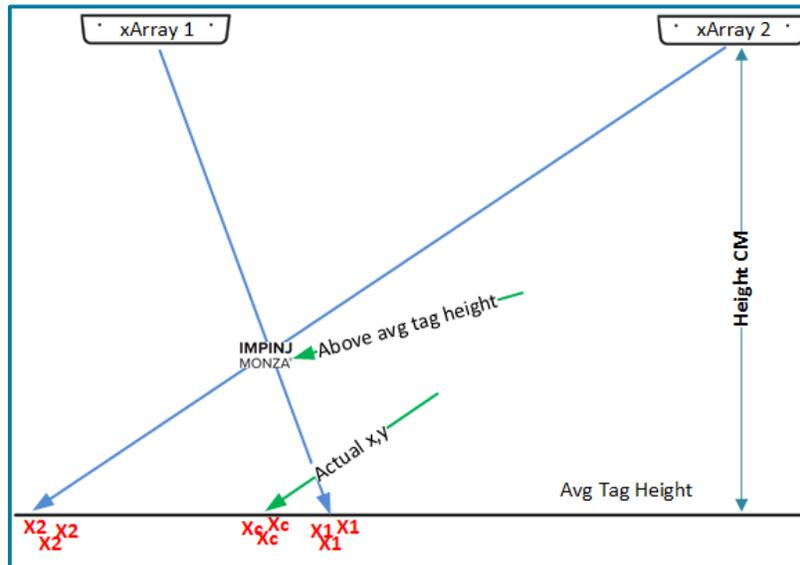
Make sure when configuring the xArray you understand that HeightCM is the distance from the xArray to the average tag height. It is not a measure of the height of the xArray to the floor (unless for some unusual reason you are trying to read tags lying on the floor). The distinction is highlighted in Figure 39. Tag heights will usually vary considerably, so you likely have to do a best guess *estimate* of the average tag height.
