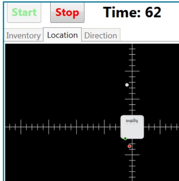
*ItemTest Location Mode showing real-time computed tag locations based on last calculated location*
