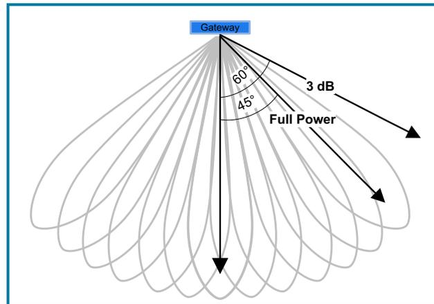
Enabling all 52 antennas of the xArray provides a circular 3 dB beamwidth coverage area of approximately 120°. In other words, the xArray will transmit full power - 3 dB towards a tag that is offset by 60° from directly under it. Figure 4 shows the xArray's circular coverage area.
