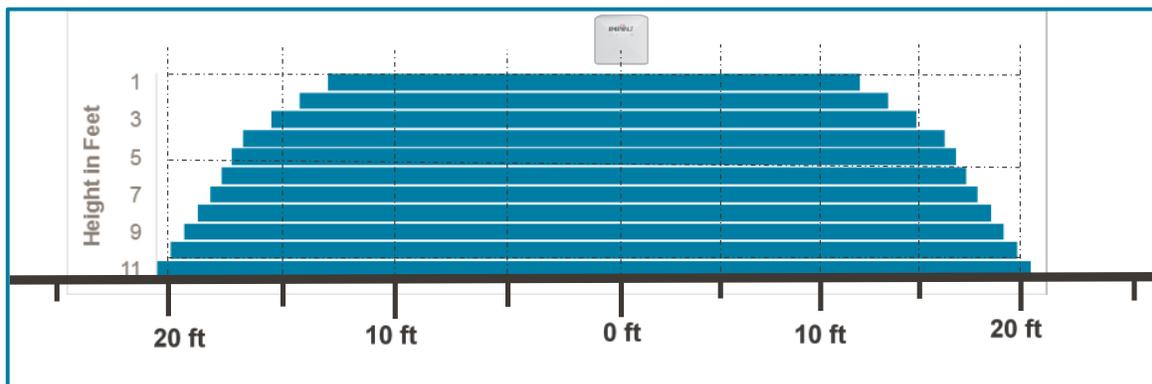
Table 4 shows the dimensions of xSpan’s oblong coverage based on  $\geq 90\%$  unique tags read using 70mm Monza R6 tags in free space. Figure 7 and Figure 8 represent the coverage area of the xSpan over height along the major and minor axes, respectively.
