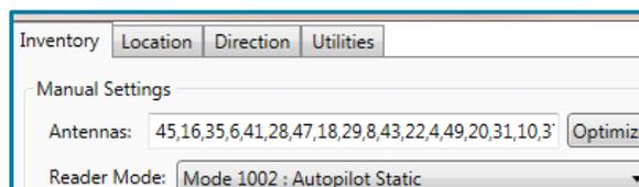
Click *Optimize* to generate a field-tested, high-performance alternating antenna sequence. The specific firing order is shown in the *antennas: edit box*. *ItemTest* dialog shows *Optimized antenna sequence*
