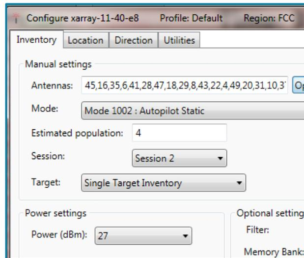
*The power setting has been reduced from max power at 30dBm to 27 dBm. Keep observing the tag reads as power is reduced to determine the amount of overdeployment.*
