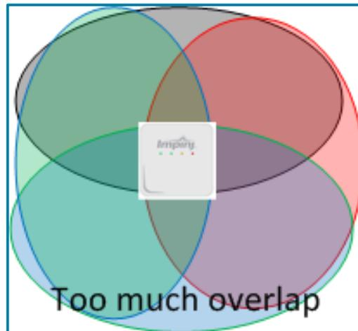
*Narrow FieldOfView produces excess overlap in Tag Direction Mode when 4 sectors are used. (xArray only)*
