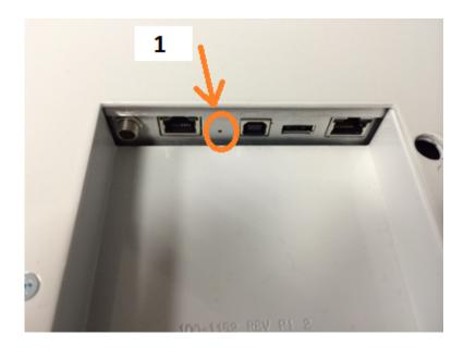
1. Default Restore Button: Insert and hold sharp point here for 3 seconds. Release before 10 seconds.
