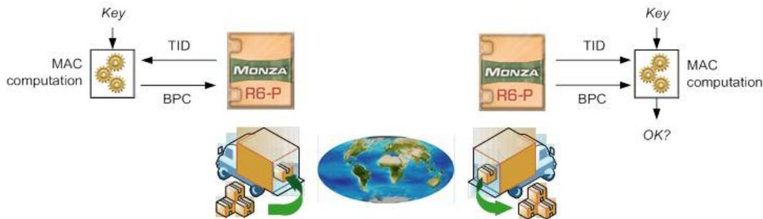
After the BPC is generated it should be written to user-memory. The BPC need not be locked/permalocked after writing, though it can be if preferred. While the contents of unlocked memory can be changed or deleted and this would cause MAC verification to fail, the cryptographic properties of a MAC are such that it is not practical to generate a false BPC for a given TID.
